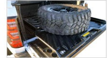
Three-Position Paused, 70% Extension, 200KG Payload Rating
